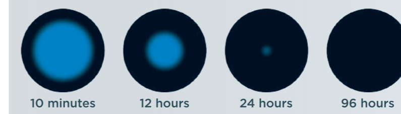
The schematic shows the setting process which is directed from the outside to the inside of the injected cement
